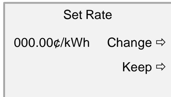
this screen. The rightmost digit of the price will be flashing. To change this digit, press the Top Button and cycle through the numbers 0-9 until the desired value is displayed. Then press the Bottom Button to save this digit. The next digit to the left will then be flashing. Repeat the process until all five digits show the desired values. After the last digit is saved, your **EMU-2™** will go to the *Time Options* screen.
