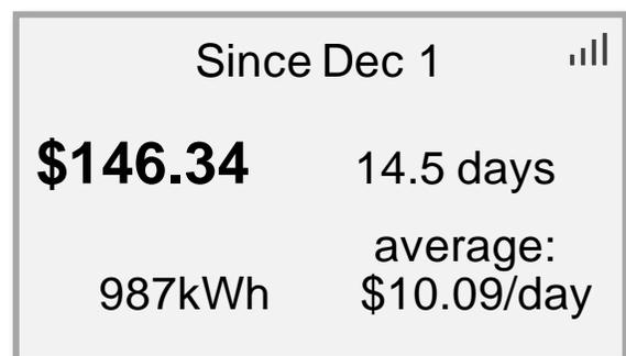
consumption for the time period is shown as recorded by the smart meter. The estimated cost for the recorded energy consumption is shown in dollars (or cents, if it is less than one dollar), and is based on the current price value during the period. The average cost per day for the current time period is shown in the lower right of the screen.
