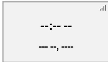
As soon as the dashes are replaced with the current time and date, it means that your **EMU-2™** has successfully read the meter, and is ready for use.
